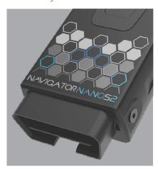
16 Pin OBD Connector Wireless Bluetooth 5.0 High Speed 2.0 USB C
