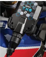
16 Pin CPC Connector Wireless Bluetooth 5.0 High Speed 2.0 USB C
